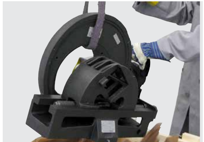
Lift the machine with a crane (or similar lifting equipment) out of the transport crate and supply it again.
