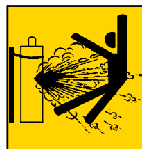
GAS CYLINDERS Shielding gas cylinders contain gas under high pressure. If damaged, a cylinder can explode
