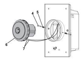
5) Connect the new motor to the motor cables (7). Mount the motor in the same position as the old one.
