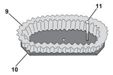
8) Mount the complete spark filter to the separator plate. Fasten with the supplied M6 nut (12).
