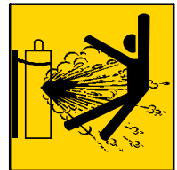
GAS CYLINDERS Shielding gas cylinders contain gas under high pressure. If damaged, a cylinder can explode
