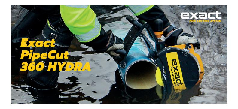
A revolutionary pipe saw that delivers excellent cutting results in wet, even underwater conditions with exceptional safety. The required power can be sourced from a compact hydraulic power pack or an excavator, making it operable in locations even outside the electrical grid.
