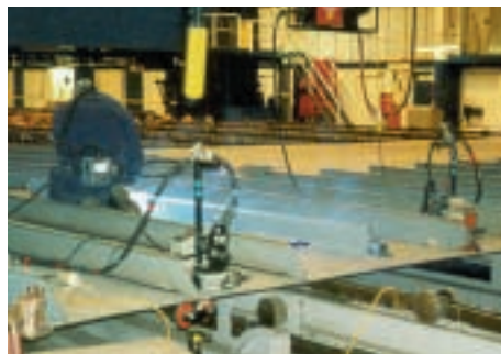
Above: Stiffener welding using Gullco Moggy trackless fillet welding machines.
