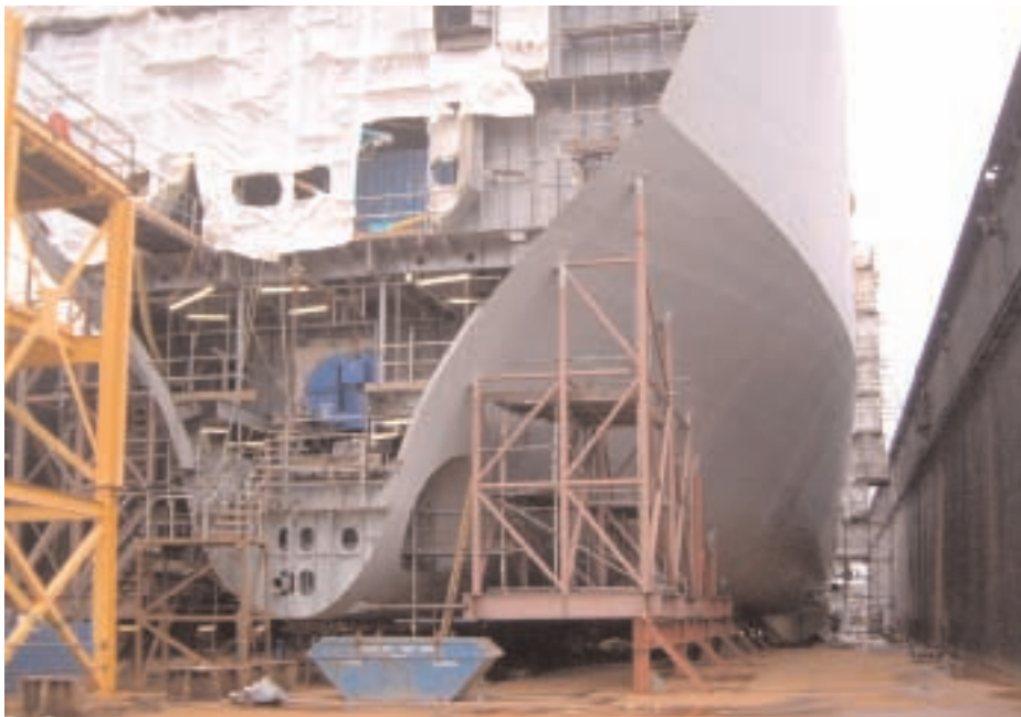
Alternative Landing Naval Ship under construction at Swan Hunter Tyneside Ltd. shipyard in Wallsend, England. When complete the ship will have an overall length of 176.6 m, a 26.4 m beam and deep displacement of 16,000 tons.
