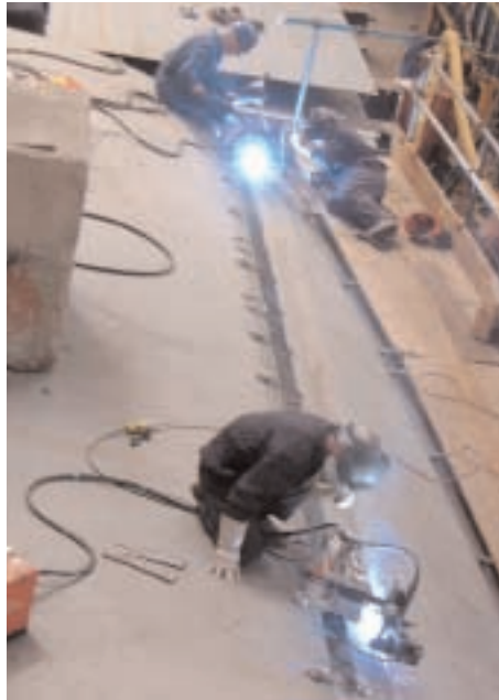
Gullco Kat Travel Carriages are used extensively to produce quality welds in all positions at the Swan Hunter Shipyard. Coupled with Gullco Oscillators, these units produce high quality mechanized welds in good production times.
