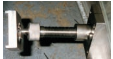
Above: close-up of clamping assembly and right: swivel mechanism. A section of the track ring is visible in the bottom left of the picture.
