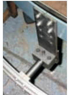
Above: close-up of clamping assembly and right: swivel mechanism. A section of the track ring is visible in the bottom left of the picture.
