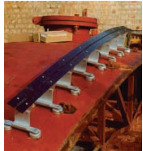
Below: Strong backs with cut outs for KATBAK ceramic weld backings are used to provide 100% X-ray quality weld from one side.
