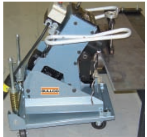
Gullco series of GBM Plate Edge Bevellers provide clean machined bevels in preparation of welding.
