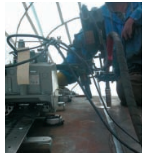
Above: Gullco Flex Kat Oscillator Combination runs on Gullco flexible track held in position using magnetic mounting assemblies
