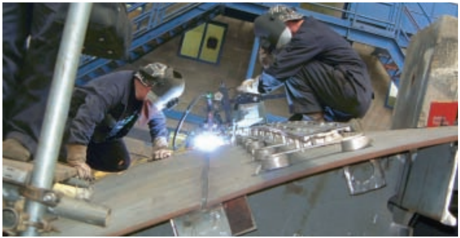
Single sided welds were possible in many weld operations through the use of Gullco KATBAK ceramic weld backings. This improves weld quality and reduces weld time by as much as 50%.
