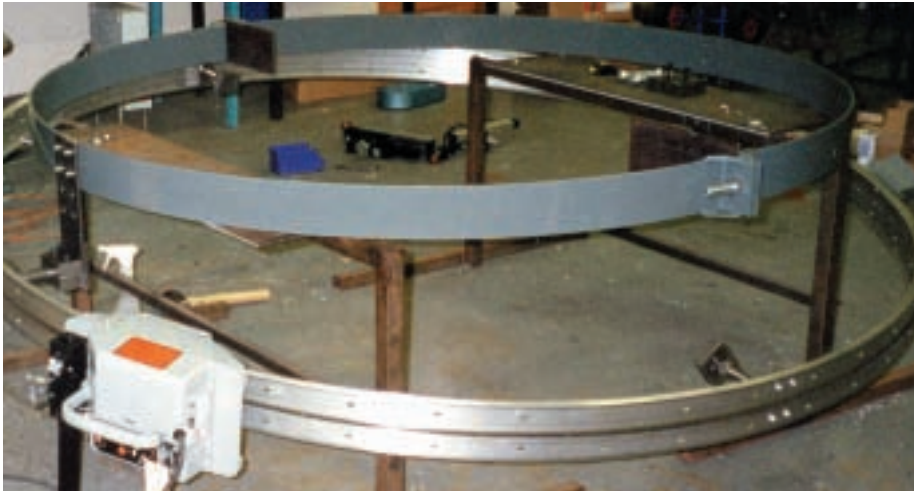
Above: One of the 1.9 m rings during manufacture with the KAT Travel Carriage fitted on the formed KAT track ring. The ring is suspended from the steel bands via swivel mechanisms.
