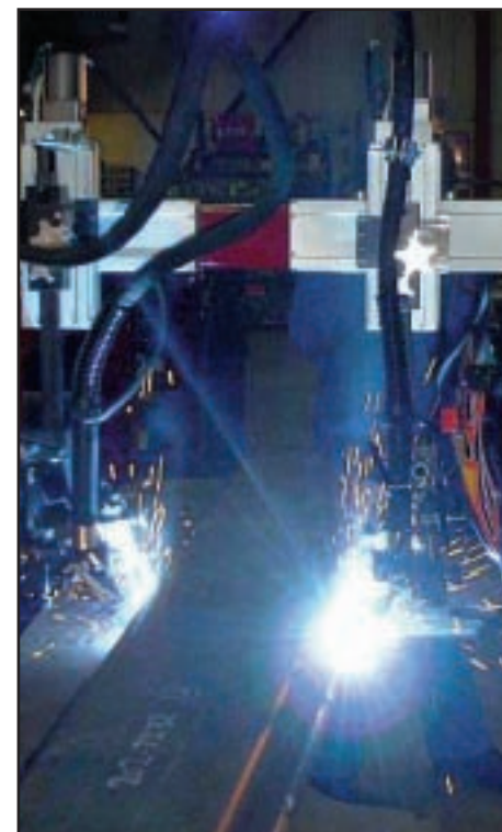
Above: Dual torches guided by Gullco Kat-Trackers simultaneously weld both sides of the work piece.
